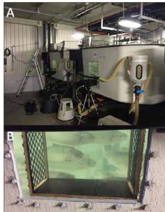
Fig 5.14. The two 3.3 m 3 tanks at Nofima Center for Recirculation in Aquaculture with plexiglas windows used for the testing of the AkvaVision system in RAS (A). The wooden frame was added to the tanks when the AkvaVision system was placed outside the tank (C).
