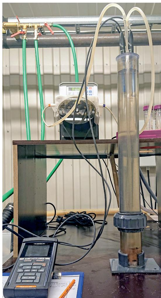
Figure 4.5. Testing a sediment reactor prototype. Photo: Andre Meriac/Nofima.
