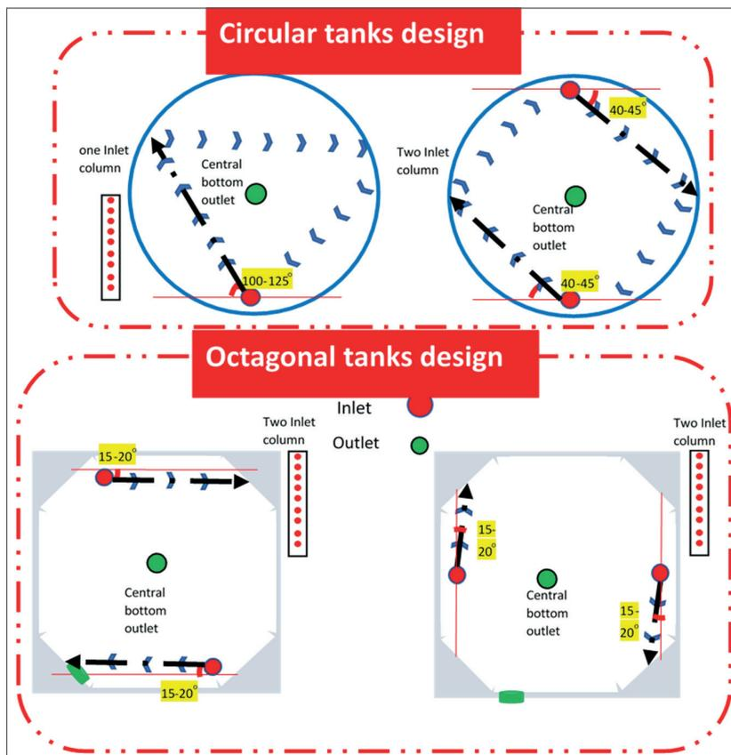
Figure 4.7. Recommended orientation of inlet column nozzles for circular tanks with one or two inlet pipes and octagonal tanks with two inlet pipes.
