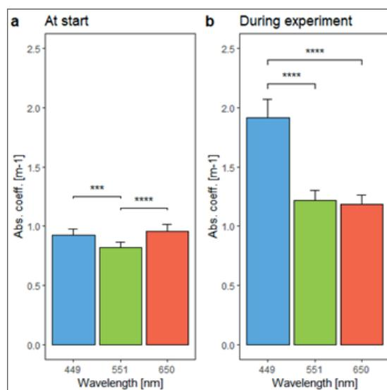
Figure 4.1. Differences in the absorbance of different wavelengths in RAS. Once feeding has started, the absorbance characteristics of the water changed, increasing the absorption of blue light and thereby reducing its transmission in the water of the tanks.
