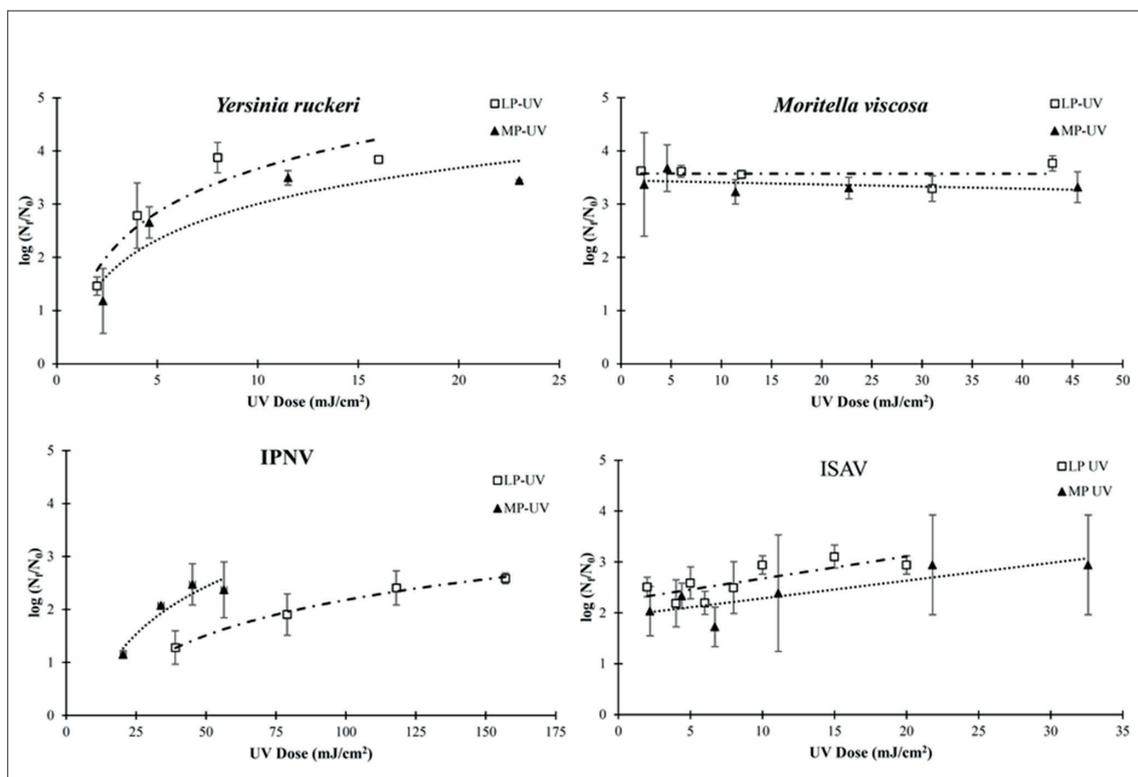
Figure 4.8. Dose response curve for inactivation of *Yersinia*, *Moritella viscosa*, IPNV and ISAV exposed to various doses of LP-UV and MP-UV irradiation.
